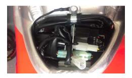
Separate all connectors and make sure they are pushed together correctly. Secure with small cable ties or tape. **ENGINE 2T**
