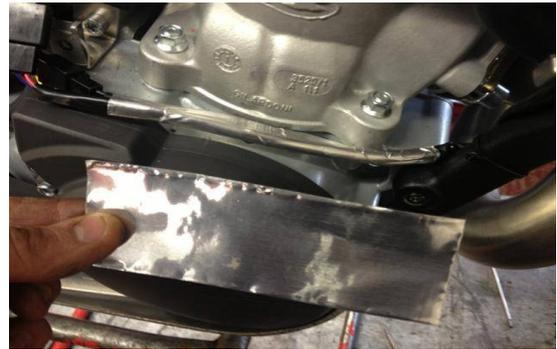
**MUD FLAP + TAPE** Very important. Fit well before so you know it works correctly. Prevents mud from clogging up the radiator. Also run some Gorilla tape (this is stronger than standard duct tape) down the back of each side of the front fender, about 2cm out of the side of the back of the fender. Fit so mud flap nuts are under the mudguard as sometimes they can flick off the radiator cover (rivet would be better).
