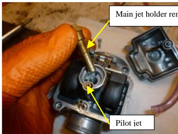
The main jet holder bottoms on the needle jet in the body of the carb. This jet does not normally come out, but it has been known, so make sure you do all the work on a clean bench, and check that the brass jet, seen in the centre of the bore below is still there when you come to reassemble! Symptoms of missing needle jet, ticks over ok, but will not rev out.
