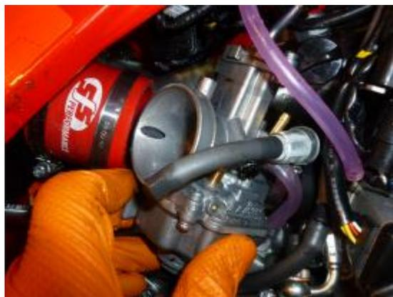
Have some paper towel ready so that when you drop the carb away from the top cover, the slide has something clean to rest on. Wipe/blow off any dirt from the carb body before slackening the bottom screws to allow trapped fuel to escape then move to the bench to remove the bowl. The carb needs to be inverted so that the brass overflow pipe fitted to the bowl will not foul the floats
