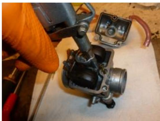
When handling the carb be careful not to squeeze the floats together as the brass overflow tube fitted to the carb bowl has to pass the inside of the left float during fitting of the float bowl. Again keep the carb body inverted to fit the bowl and after assembled, give it a gentle shake up and down so that you can hear that the floats are free to move.
