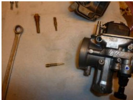
Blow through the airscrew & pilot jet holes as they allow the mixing of fuel and air for low throttle openings and are often overlooked resulting in poor carburetion. Blow through the hole for the main jet holder and the removed pilot & main jets before refitting.
