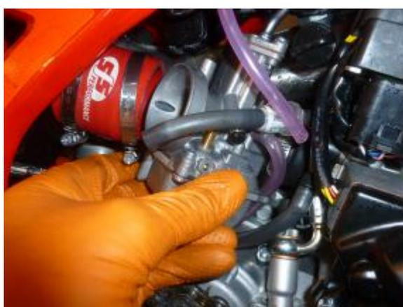
Refit the carb body to the slide, fit the top screws, offer the carb up to the engine side whilst gently pulling the throttle cable through from the top of the tank then twist the carb into position. Connect up the vent and fuel inlet pipes and slide the carb inlet tube forward and secure. Poke the small overflow pipes down through the wire guide under the carb and down behind the gearbox.
