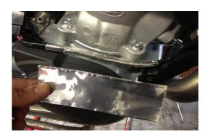
**MUD FLAP + TAPE** Very important. Fit well before so you know it works correctly. Prevents mud from clogging up the radiator. Also run some Gorilla tape (this is stronger than standard duct tape) down the back of each side of the front fender, about 2cm out of the side of the back of the fender. Fit so mud flap nuts are under the mudguard as sometimes they can flick off the radiator cover (rivet would be better).
