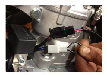
**FAN WIRING** If you do remove any wiring from your bike please contact us. Do not remove any electrical boxes or change any wiring. The fan is wired through the lighting loom/wires on a standard bike.
