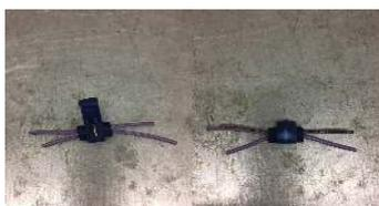
Electrical adaptor to wire the fan live if the fan wiring/thermostat fails. Available from us. Get before the event. This is very good to carry.
