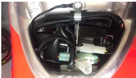
Separate all connectors and make sure they are pushed together correctly. Secure with small cable ties or tape.
