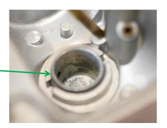
To check amount to machine off - take out sealing o-ring and fit plug to bowl. Looking for a flush level with the boss in the bottom of the bowl
