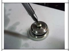
Now you need to put in the next piston. But first remove the screw and "O" Ring from the centre, so as you put it in the cartridge air can escape through the centre.
