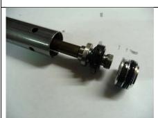
Then carefully pushing down on the rod you will remove the sealing piston. This has a Teflon strip around it's perimeter – check for wear and replace if necessary.
