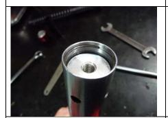
If doing a complete disassembly turn the cartridge upside down and push down on this bush to reveal the retaining clip. Remove with small pick or similar. Be careful not to send it flying across the workshop as it is released!
