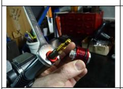
Carefully remove it in an upward direction, being careful not to damage the internal adjust rod.
