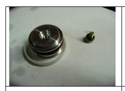
Once it is just under the surface of the oil (a few centimetres down from the lip edge), then screw the centre screw and "O" Ring back in. It should now be fully primed and you can put in the bottom out spring, bush and retaining clip so the cartridge is completely reassembled.
