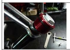
Now using a 17mm open ender for the lower nut, and a 14mm thin open ender for the top nut remove the fork cap.
