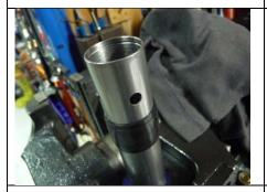
I wrap a bit of Rescue Tape around the small bleed hole to stop the loss of oil from this orifice whilst filling.
