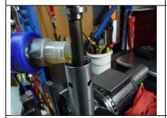
IMPORTANT NOTE: When reassembling, these fork cartridges must be FULL of oil – NO AIR at all, or you will get erratic damping, and a nasty top out "CLUNK" on extension.
