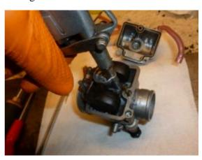
When handling the carb be careful not to squeeze the floats together as the brass overflow tube fitted to the carb bowl has to pass the inside of the left float during fitting of the float bowl. Again keep the carb body inverted to fit the bowl and after assembled, give it a gentle shake up and down so that you can hear that the floats are free to move.
