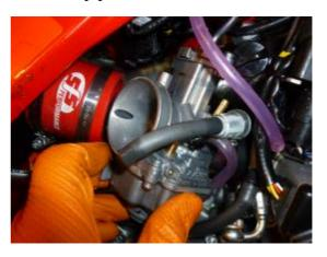
Have some paper towel ready so that when you drop the carb away from the top cover, the slide has something clean to rest on. Wipe/blow off any dirt from the carb body before slackening the bottom screws to allow trapped fuel to escape then move to the bench to remove the bowl. The carb needs to be inverted so that the brass overflow pipe fitted to the bowl will not foul the floats
