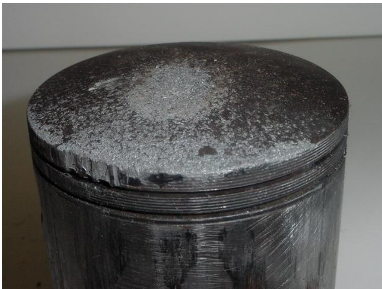
Two-Stroke Piston Showing Detonation Damage
