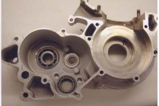
Clean all gasket surfaces using a razor blade.
