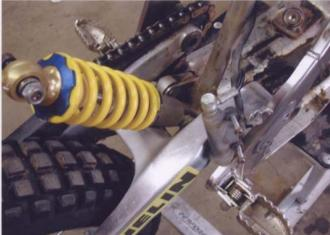
After engine removal with swingarm pulled back.
