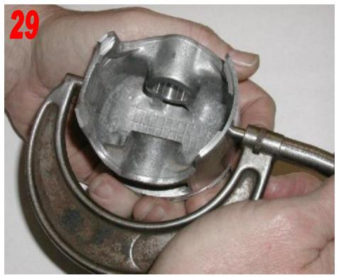
→ Using an outside Micrometer carefully measure and record the diameter of the piston.
