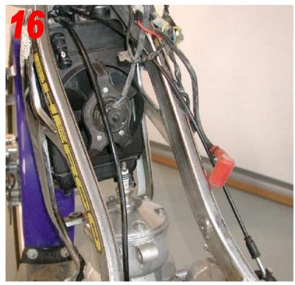
→ Slide the radiator up in the frame. This provides clearance to remove the cylinder.
