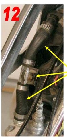
Using a pair of pliers release the hose clamps on the radiator hoses.
