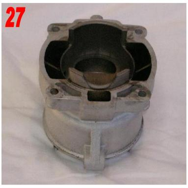
This photo shows the cylinder base cleaned and ready to be reinstalled.
