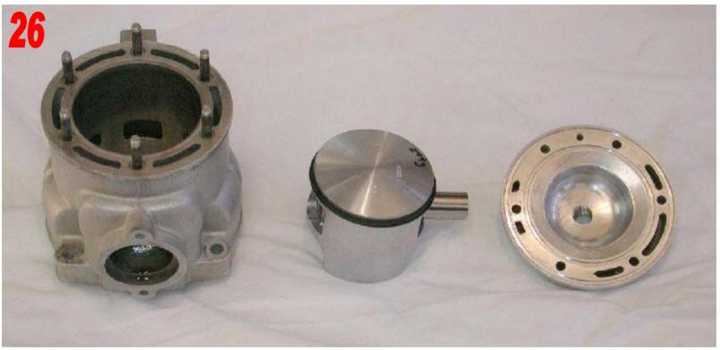
This photo shows the cleaned cylinder, cleaned piston (new in this case) and the cleaned cylinder head. The threads on the cylinder head mounting stude have had the rust removed.
