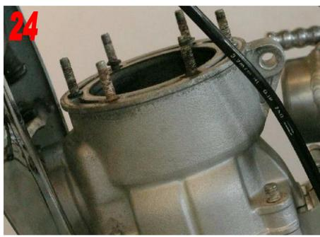
→ Using a 13mm Socket remove the 4 nuts that hold the cylinder to the case.
