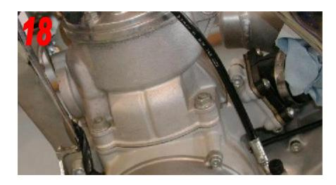
Using a 13mm socket or box end wrench remove the 4 bolts that retain the cylinder to the case.
