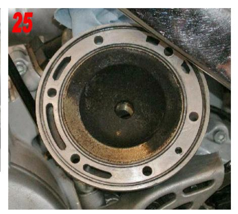
This photo shows the inside of the cylinder head and the 2 O-ring seals. There is a light coating of carbon that needs to be removed.
