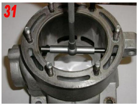
→ Use a telescoping gage to measure the cylinder bore.
