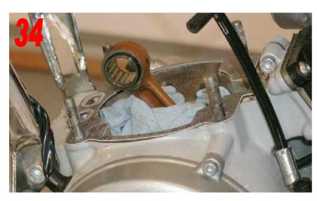
Install a new base gasket onto the engine case. Handle the base gasket by the edges and do not allow your fingers to transfer oil to the gasket, this will help insure a good seal.
