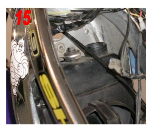
Remove the radiator mounting bracket.
