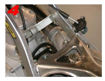
Remove the fuel tank and the air box.
