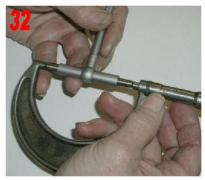
Use the exact same micrometer that was used to measure the piston O.D., measure the telescoping gage to determine the actual cylinder I.D.
