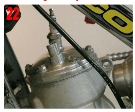
This photo shows the cylinder head and the nuts that must be removed.
