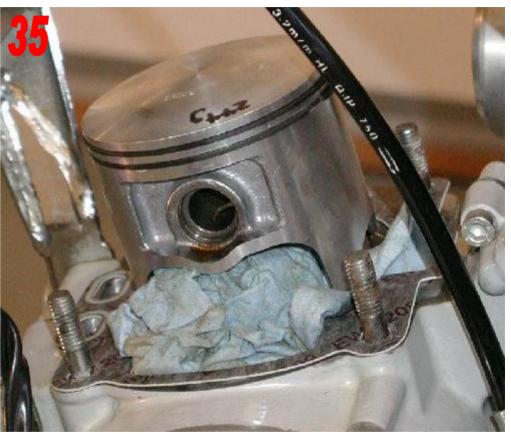
Install the piston onto the connecting rod, make sure that the arrow is facing forward. Push the piston pin all the way into the piston and install the remaining circlip.
