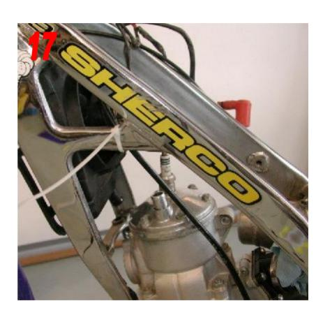
Using a zip tie attach the clutch line to the frame.
