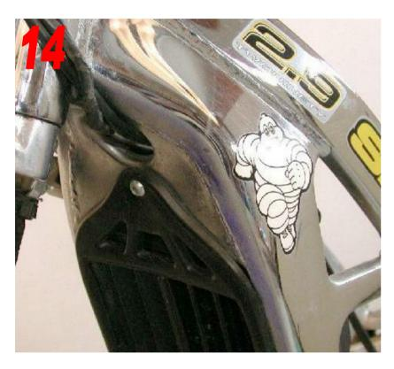
→ Using a 4mm Allen Wrench remove the radiator mounting bracket bolt.
