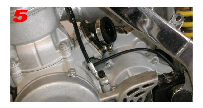
Remove the carburetor. Not required but recommended.
