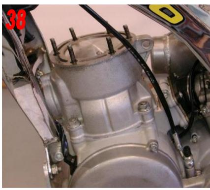
Seat the cylinder onto the engine case and install the 4 nuts. Tighten these nuts to 16 ft lbs (2,2m/kg)
