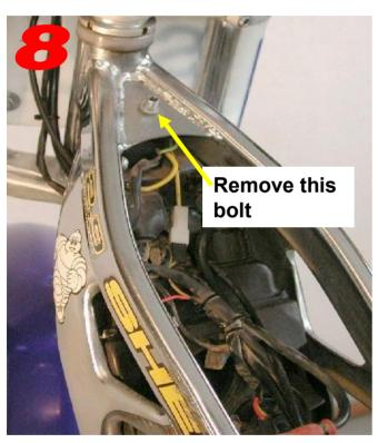
Using a 12mm socket or box end wrench remove the bolt that holds the coil assembly to the frame.
