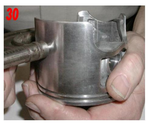
The piston and micrometer should be held as shown, the measurement should be taken across the skirt of the piston 3/4" (19mm) from the bottom of the piston.
