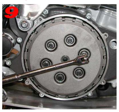
Using an 8mm socket carefully remove the 6 bolts that retain the clutch springs. Loosen the first bolt a few turns and then go to the next bolt. The bolts should be removed in sequence.
