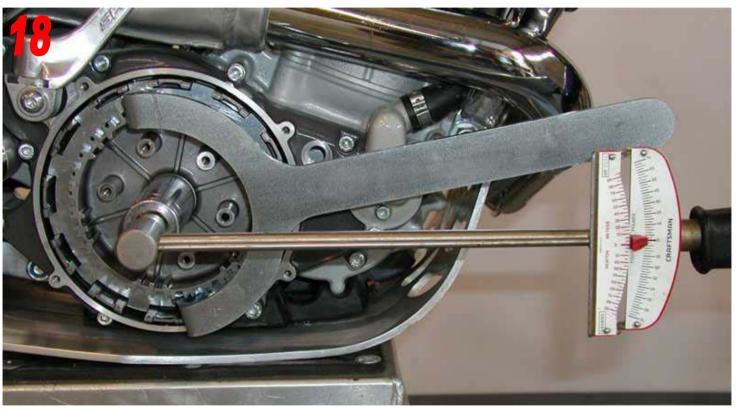
→ Using a 24mm socket, a good quality torque wrench and the RYP Clutch Holder Tool tighten the clutch hub retaining nut to 45 ft lbs (60 Nm).
