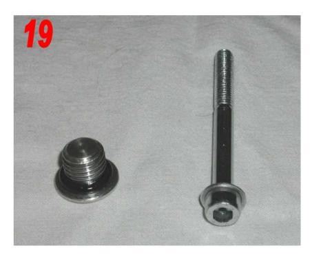
Inspect the transmission filler O-ring and the transmission drain sealing washer, replace if damaged
