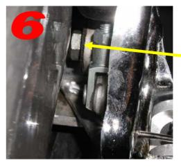
Locate the rear brake pedal mounting bolt.
