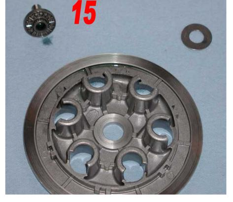
Photo of the clutch assembly with the spring holder removed. Note the location of the clutch release bearing.
