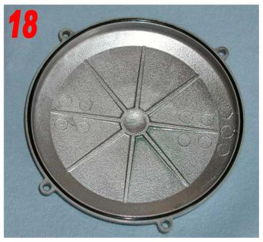
Inspect the clutch cover O-ring, replace if damaged.
