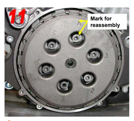
In order to make sure that all of the parts are reassembled in the same location as they were removed from, use a felt tipped pen and number the clutch spring holder as shown.
