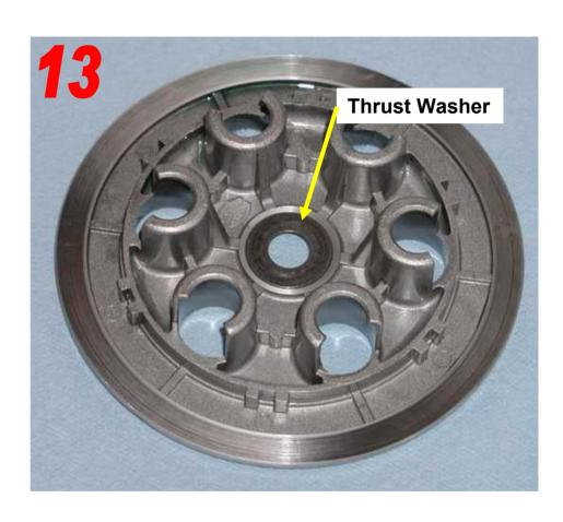
Clutch spring holder. Note the thrust washer location. The thrust washer stuck to the spring holder as it was removed.
