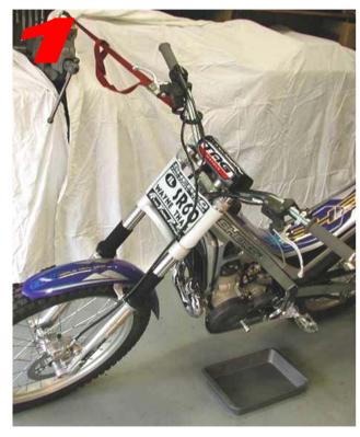
Lean the bike over in order to drain the transmission fluid, this method works well for the author.
