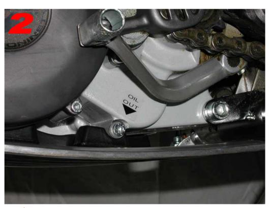
Locate the transmission oil drain screw on the left side of the engine, behind the gear shift lever.
