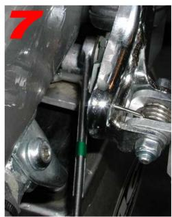
Using a 13mm box end wrench, remove the mounting bolt and the rear brake pedal.
