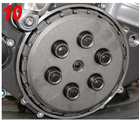
This photo shows how the bolts should be evenly removed.
