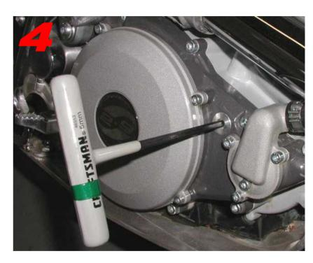
Using a 5mm Allen wrench remove the transmission oil filler plug from the RH engine case.
