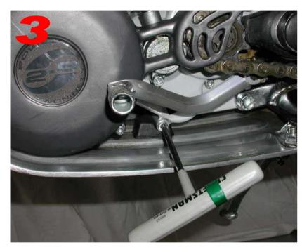
Using a 5mm Allen wrench remove the oil drain screw. Drain the oil into a suitable container. Dispose of the used oil according to local regulations.
