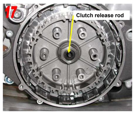
→ Using two small hooks and a magnet remove the 5 metal and 6 friction clutch discs.
