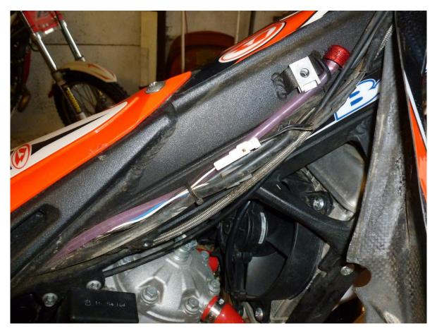
On later years, the carb vent tube goes up inside the frame so that it is protected from direct ingress
