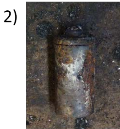
Cell vented through pre-existing vent holes at the positive terminal.
