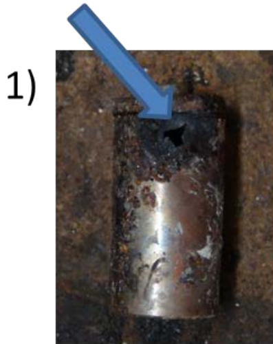
Vent holes were in alternate locations.
