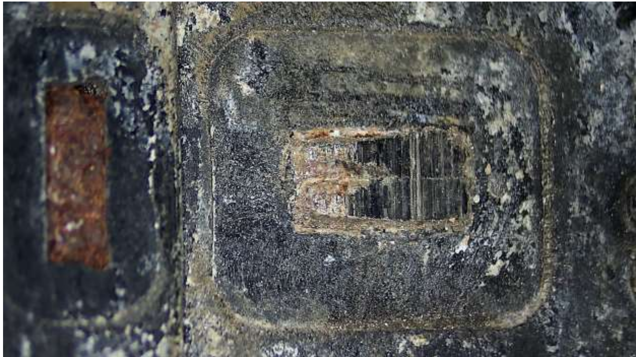
Figure 2 Close up view of the trigger module interface to the flywheel. Note the apparent wear on what I assume is a pole piece.
