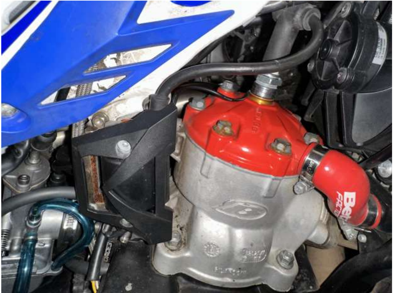
Figure 11 Temporary ground wire connected from spark plug base to ignition coil frame using a copper washer. This will be replaced with a wire from the cylinder base lug.
