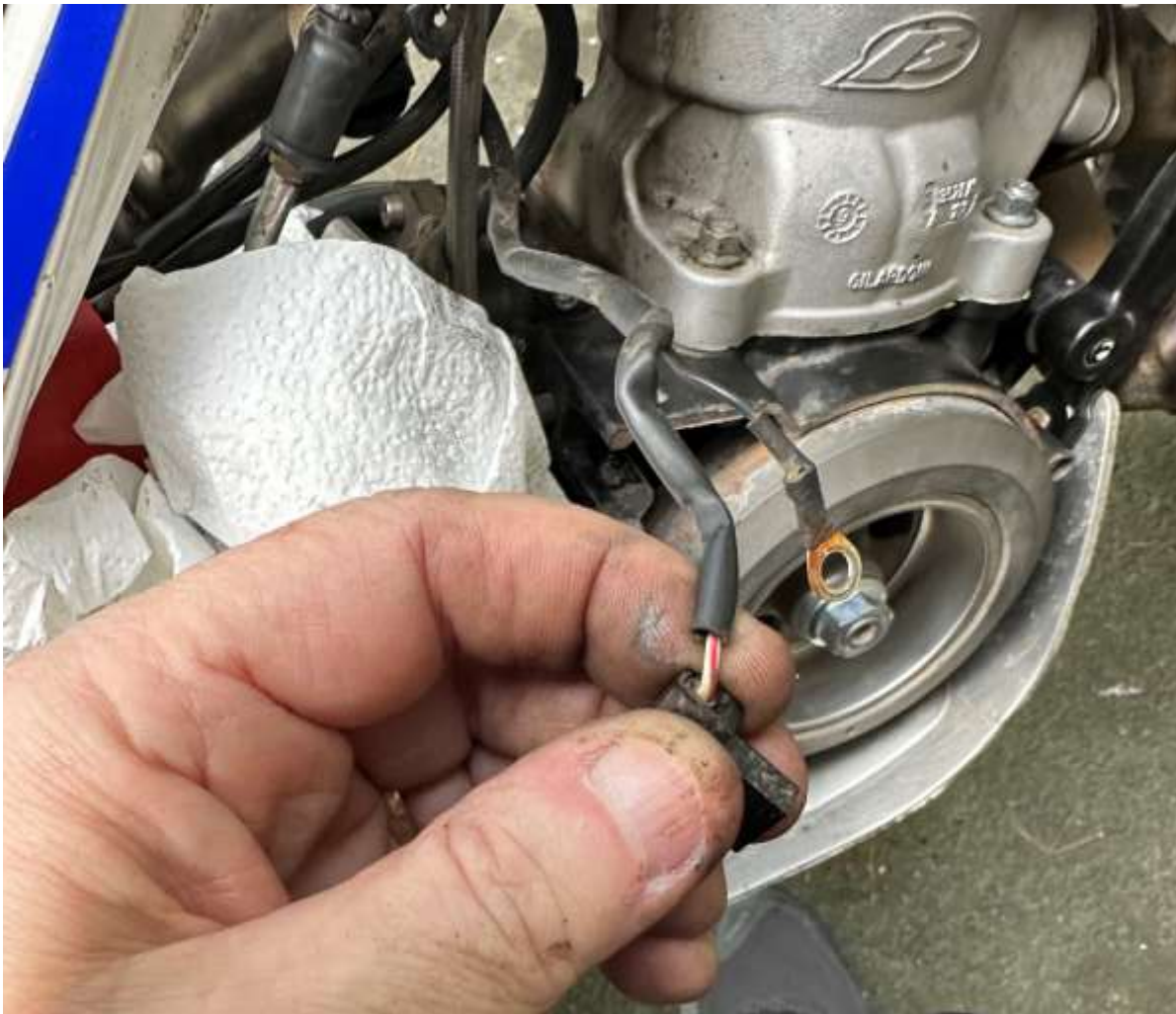
Figure 9 These are the ignition coil connections. High voltage red/white wire to spade lug and black wire to coil frame from ground nexus.
