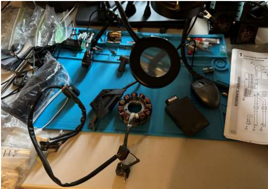
Figure 5 Ignition coil, Stator W/harness and CDI (Along with bags of carb jets, microscope lens and assorted other debris. As still lifes go it's no Vermeer)
