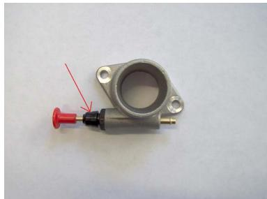
3. Widen the calibrated hole to Ø2mm
