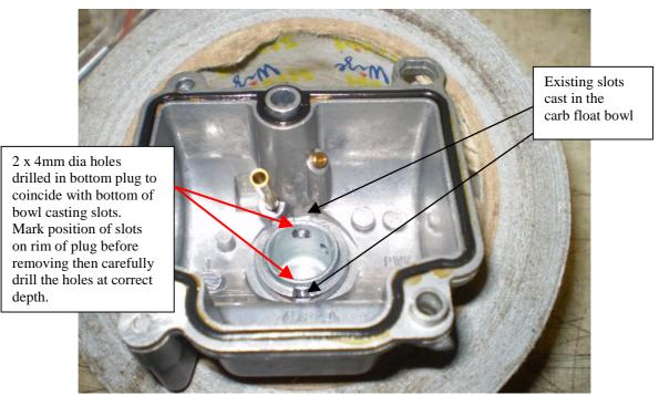
Make a mark like a saw cut on the outside of the float bowl and bottom plug to give correct alignment after plug removable.
